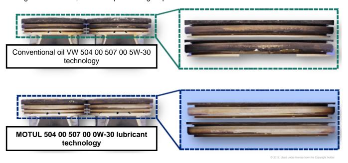
Regarding engine protection, especially wear protection, MOTUL SPECIFIC 504 00 507 00 0W-30 protects your engine as demonstrated, here on the timing system, on the VW general engine wear test 650 hours:
